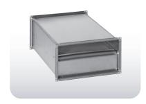
Silencers are produced using 30 mm rock wool insulation perfore sheet on the inside, aluzinc sheet metal on the outside.
